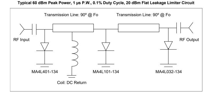
Typical 50 dBm Peak Power, 1 µs P.W., 0.1% Duty Cycle, 20 dBm Flat Leakage Limiter Circuit
